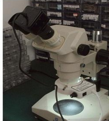
1 ) Assemble MC500 to your Microscope 2 ) connect MC500 to your PC 3 ) View, capture and record
