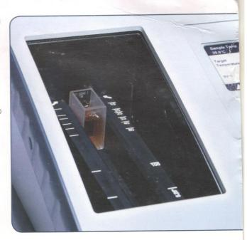
"The PFXeo solves the problem of measuring the colour of edible oils with its unique ability to not only keep the oil at a constant temperature but also to measure and report on the temperature of the sample, avoiding any misreadings from crystallization."
